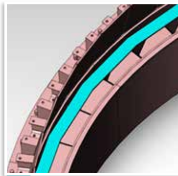
TYPICAL LOUVER RING DESIGN
